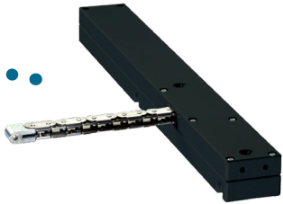
LM2 Actuators Actuators mounted on awning windows for occupant comfort. 24VDC 500mm Stroke 200N Force
