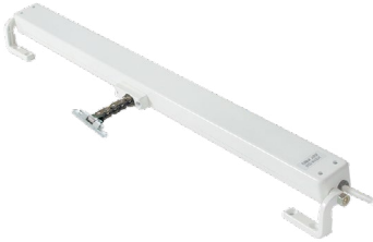
Quasar Actuators Actuators mounted on hopper windows for natural ventilation for occupancy comfort. 24VDC 500mm Stroke 300N Force
