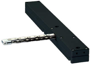
LM2 Actuators Actuators mounted on awning windows for natural ventilation in an educational setting. The system conducts night flush and maintains air exchange rates for a healthy environment. 24VDC 500mm Stroke 200N Force
