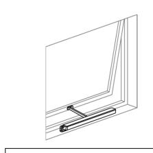
Minimum sash height is 3 times the chain length.
